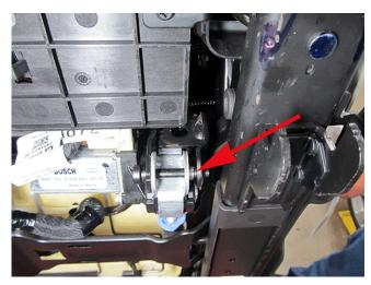
1. Locate the power seat vertical adjuster actuator attachment to the seat frame.
