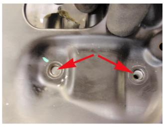
**6.** Align the holes in the seat pan with the holes in the pivots blocks.
