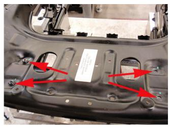
2. Remove the four screws that attach to two pivots blocks to the seat pan.
