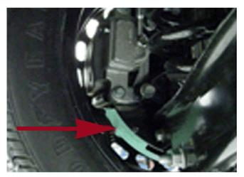
With the vehicle on a hoist, rotate the wheel while at the same time pulling the torn end of the cover away from the disc brake rotor and wheel. Ensure
