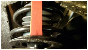
These blocks (1 per side) MUST be removed during the PDI process.
