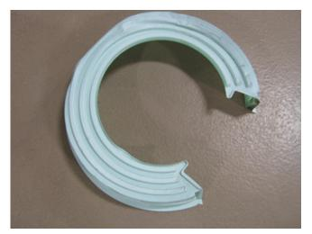
The factory installs rear disc brake rotor protection covers during vehicle manufacture. These covers MUST be removed from the rear rotors when
