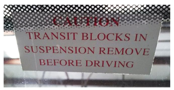
A reminder sticker to remove the transit blocks is applied to the vehicle windshield during assembly. This sticker should be removed only AFTER the transit blocks are removed.
