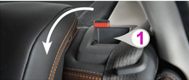
8. Reach under the safety belt and pull the lever (1) on top of the seatback. A tab near the seatback lever will raise. When the **red marking on the tab is visible**, the seatback is unlatched.
