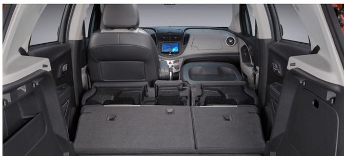
A 60/40-split, flat-folding rear seat and a fold-flat front passenger seat combine to allow storage of long items such as skis or a surfboard, up to 8 feet (2.4 m) long.
