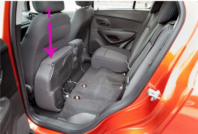
**Notice:** The rear seat cushion must be tilted forward before the seatback is folded down. Only one seat cushion is shown tilted forward in this view.
