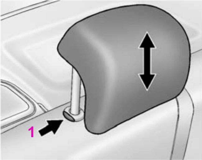
4. Fully lower the rear seat head restraint by pressing the release button (1) located on the top of the seatback and push the head restraint down.
