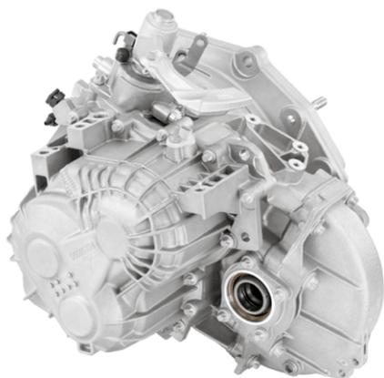
The manual 6 speed M32 transmission — RPO MR5 is used on the front wheel drive (FWD) Trax LS. All of the gears including reverse (**R**) are synchronized.
