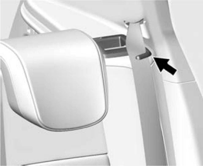
7. Make sure the safety belt is in the retainer hook on top of the seatback.
