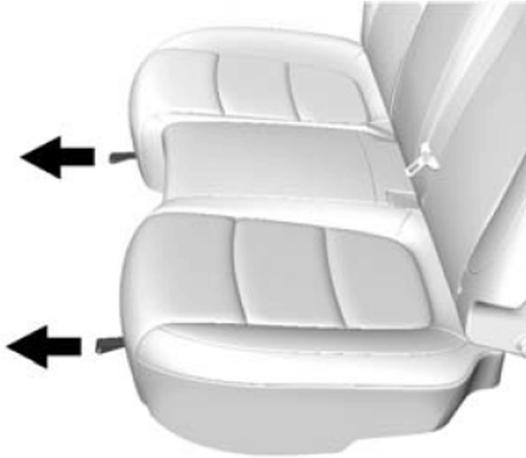
5. Pull the strap on the front edge of the rear seat cushion to release the cushion.
