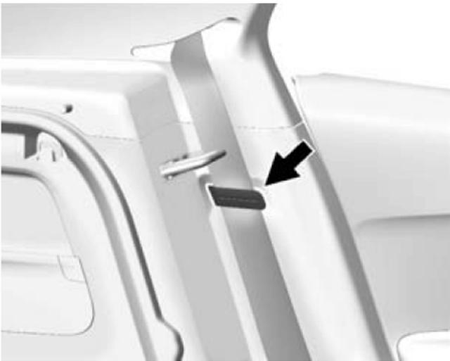
10. Place the outboard safety belt in the safety belt clip (if equipped) on the side trim of the vehicle.
