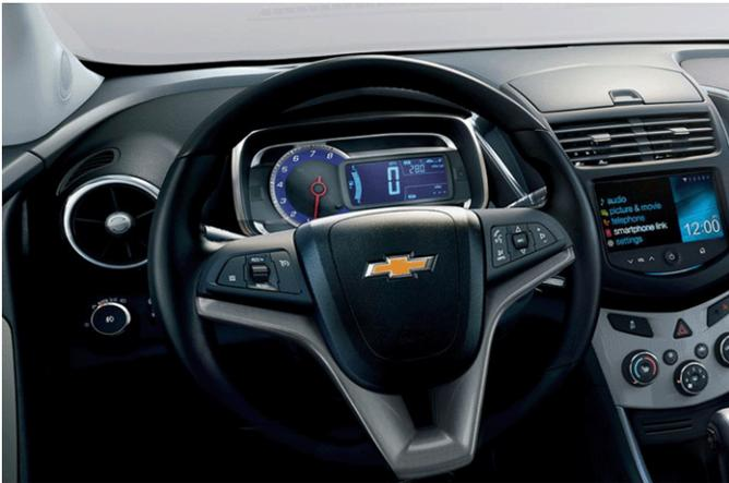
The contemporary interior environment features an instrument cluster with a large, performance style analog tachometer combined with a prominent digital display for the speedometer and other readouts. It also includes a 3.5-inch (89 mm) diagonal driver information center (DIC) display with ice blue backlighting.
