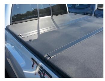
Gap from hinge cover to tonneau cover should be no more than 0 -1mm.
