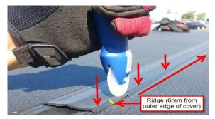
6) Run plastic pry tool below lip and pull up slightly to ensure hinge cover is properly seated.
