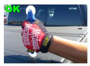
Note: this step must be performed at the position shown below, locking tab ridge (6mm from outer edge of cover), along the entire length of the hinge cover to ensure proper seating.
