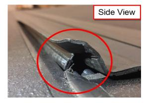
3) Spread the cover locking tab with a plastic pry tool the length of raised portion.
