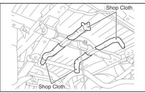
3. REMOVE THE PROTECTORS FROM THE SPARE TIRE CARRIER STOPPER
