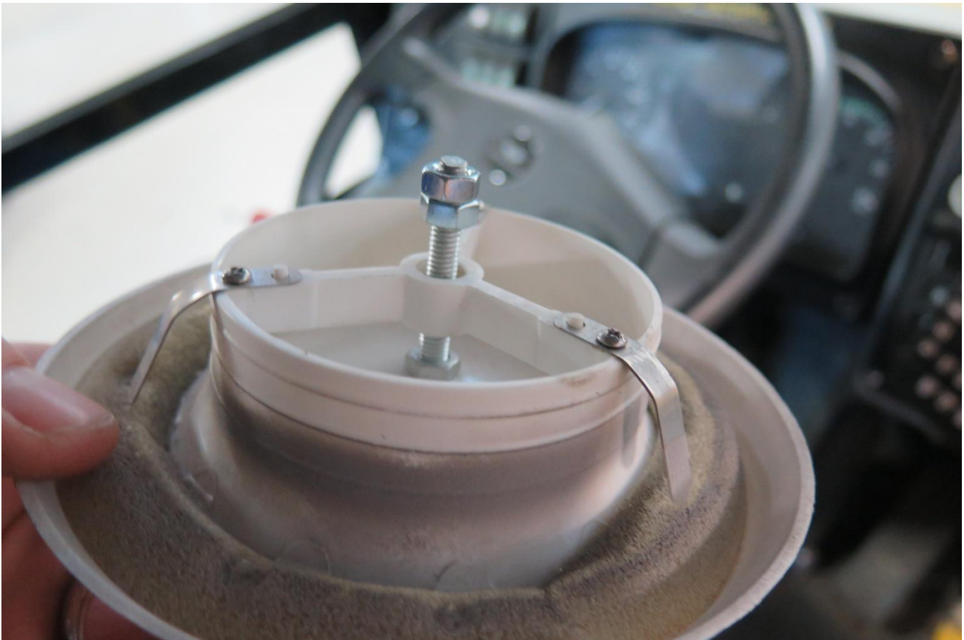
Figure 1: Adjustable Vent Removed from Socket and Reworked
