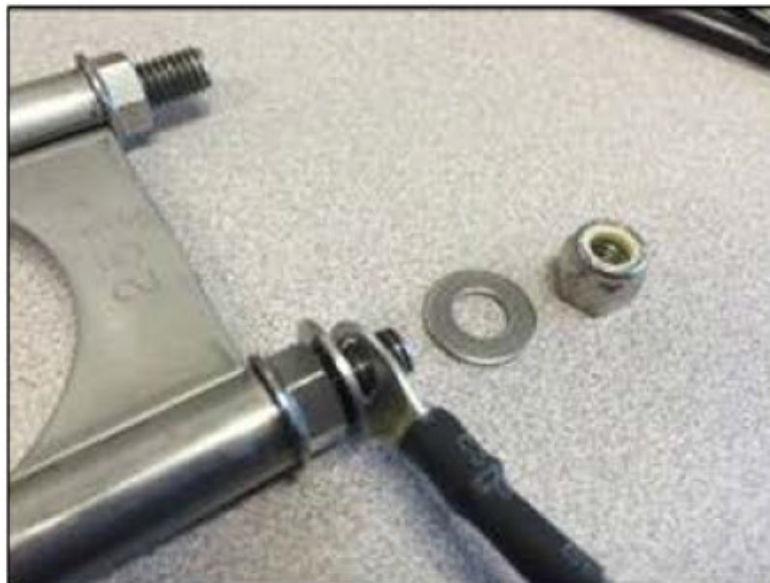
Figure 3: Ground Strap Mounting Hardware Orientation
