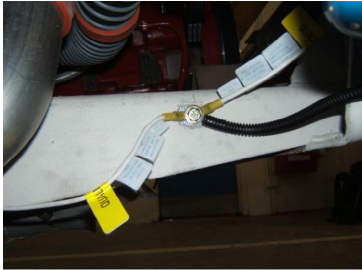
Figure 10: Common Ground Point on Bus Frame
