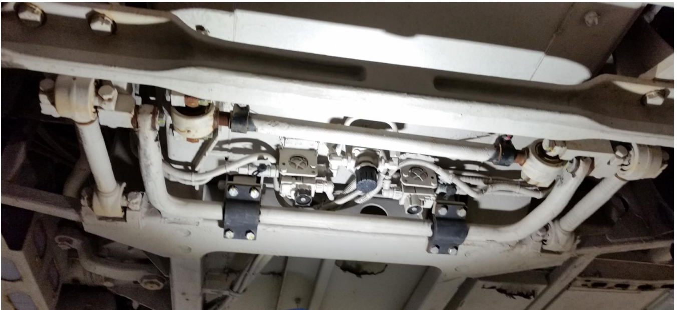
Figure 1: Sway Bar Installation.
