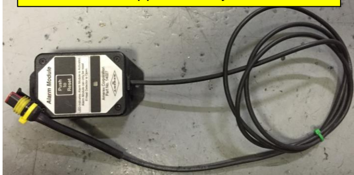
Amerex fire suppression system test tool
