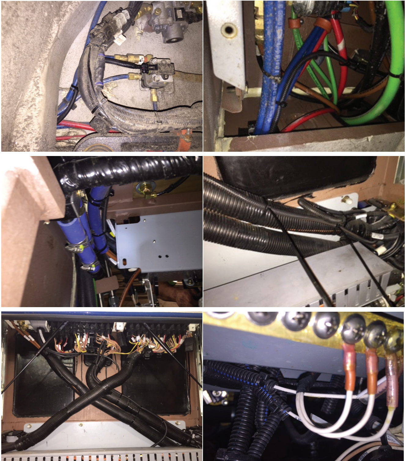
Figure 3: Front Height Sensor Cable Routing
