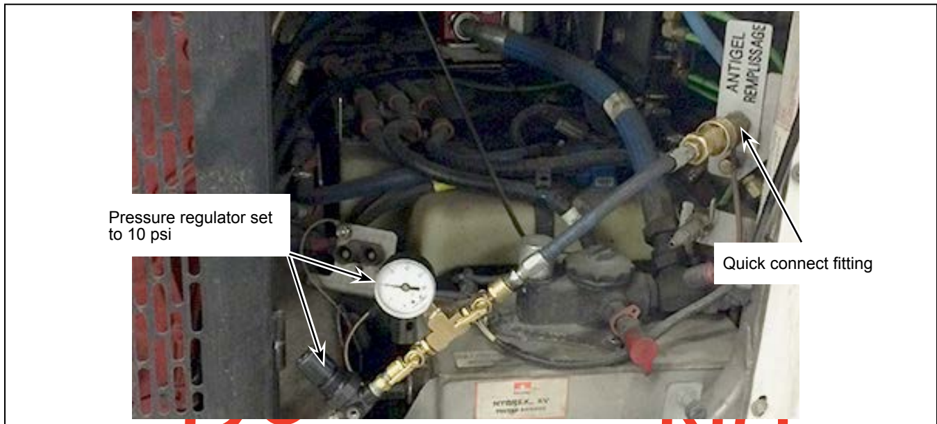
Figure 2 - Filling Hose Equipped with a Pressure Regulator
