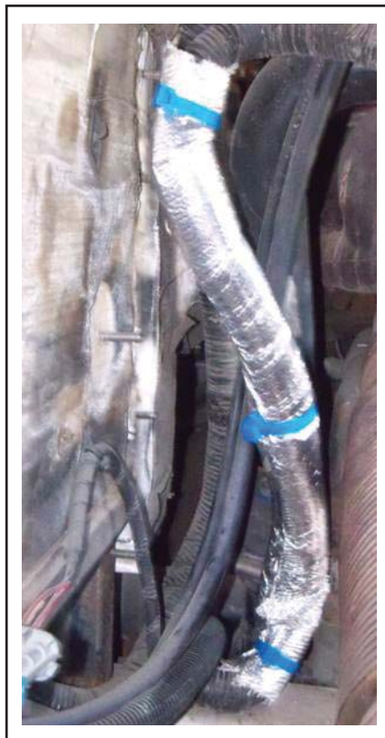
Figure 3 - Typical Heat Sleeve Installation
