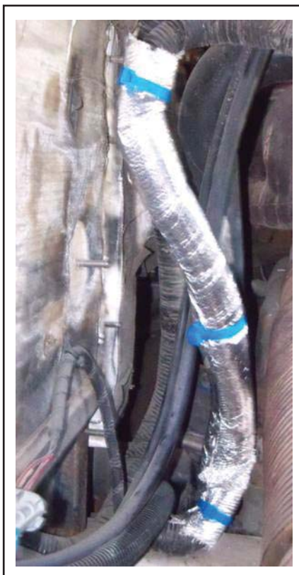
Figure 3 - Typical Heat Sleeve Installation
