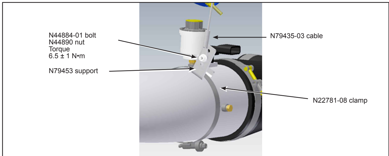
Figure 3 - Lower Support Installation
