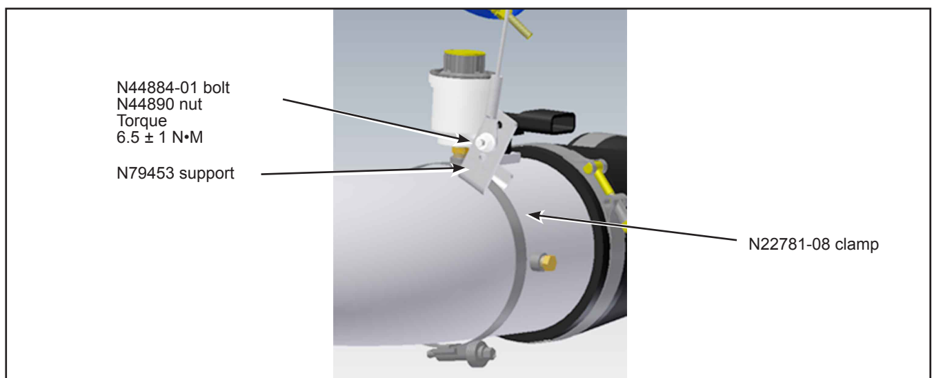
Figure 3 - Lower Support Installation
