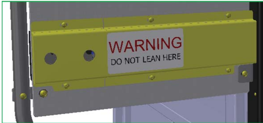
Figure 6 - Warning Decal Installation on N82084 (Partition Rear Side)
