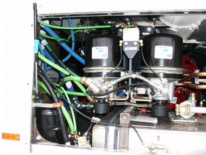
Figure 1 - Air Dryer Location
