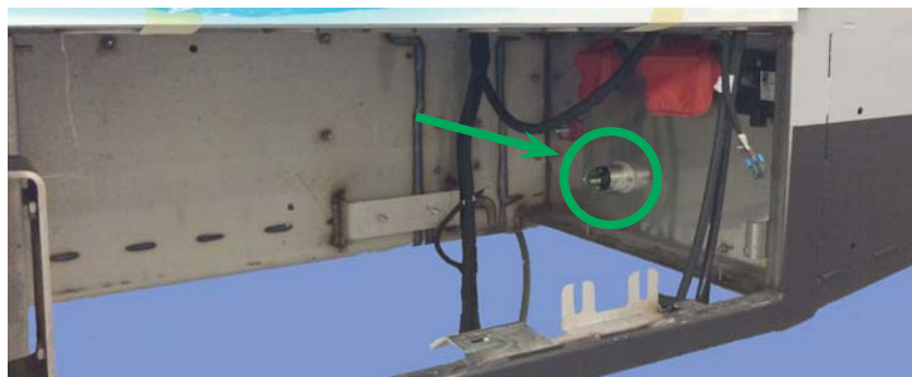
Figure 2 - Power Switch Relay Location (View from Battery Compartment)
