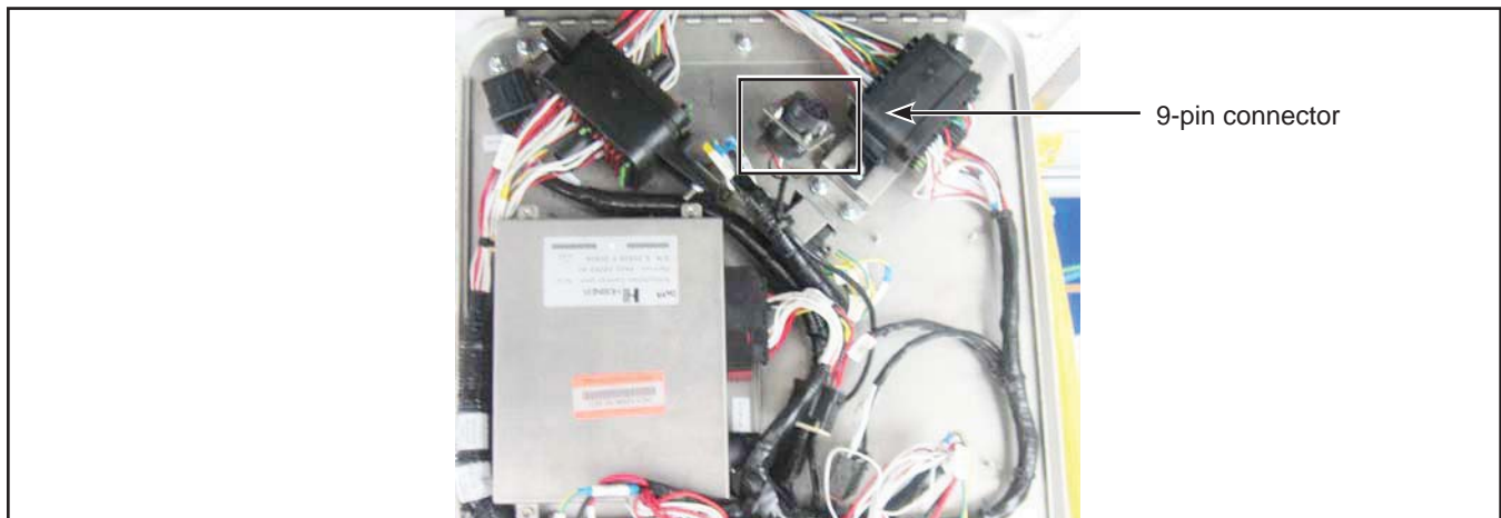
Figure 3 - RF9 Panel ACU 9-pin Connector Location
