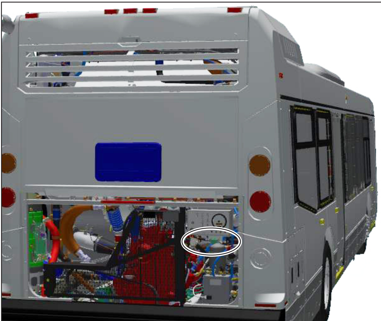
Figure 1 - Fuse Holder Bracket Location
