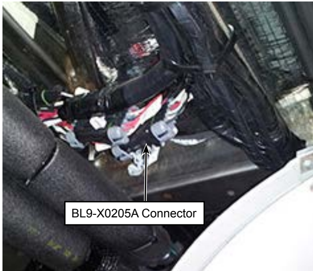
Figure 3 - BL9-X0205A and BR7-X1249A Connector Location
