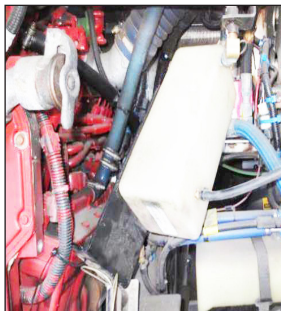
Figure 6 - Move Surge Tank Forward
