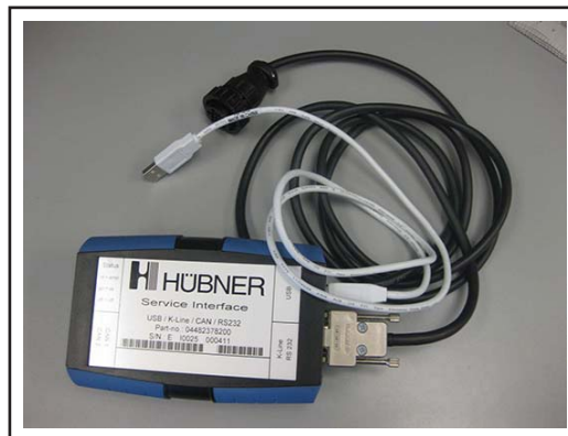
Figure 2 - Hübner Service Interface (Part N° N8900610)
