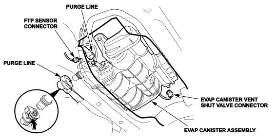
2. Remove the EVAP canister assembly by removing the three bolts.
