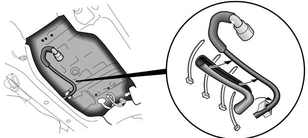
• Equally space the zip ties, and tighten the ties so that the locking tab is oriented on the top as shown.
