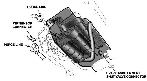
10. Using the HDS, clear the DTCs, then do the EVAP system function test.
