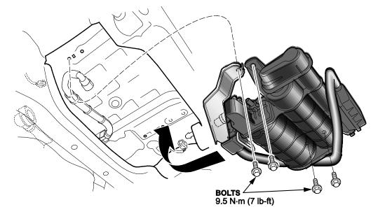
9. Connect the purge lines, the EVAP canister vent shut valve connector, and the FTP sensor connector.
