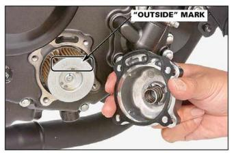
If it's your first time servicing one of these models, be sure to source the filter by *part number*, refer to the *Maintenance* section of the model specific Service Manual, follow the instructions exactly, and pay attention to the marks on the filter. As noted in the Service Manual, installing the oil filter backwards will result in severe engine damage.
