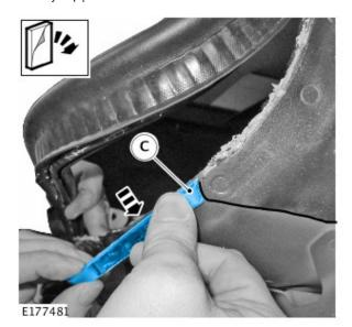
14 NOTE: make sure the seal pad is completely adhered to the vehicle.
