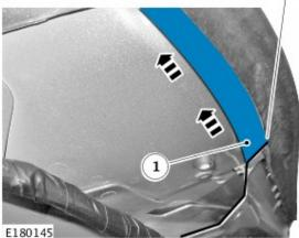
18 NOTE: the foam strip supplied will be precut to the correct lengths.
