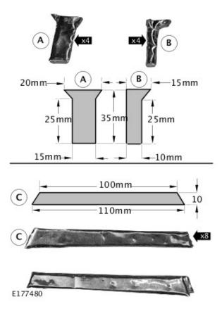
${f 10}{f S}$ tick two equal pieces together to make each piece twice the thickness.
