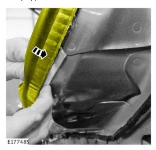
16 NOTE: make sure the tailgate weather strip completely covers the seal pad when installed.
