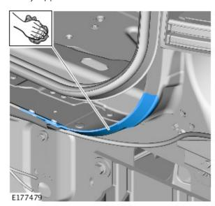
12 NOTE: make sure the seal pad is completely adhered to the vehicle.
