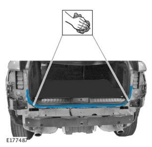
**7**Use a suitable tape to wrap the rear electrical harness.
