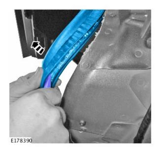
**9**Use a suitable tool to cut the seal pad to the sizes shown.
