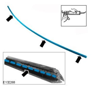
4Install the upper windshield finisher, ensuring it is located properly.
