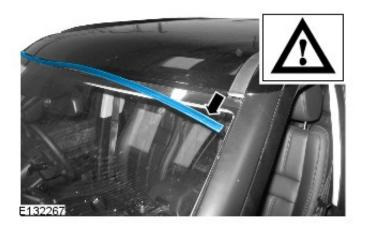
2 NOTE: make sure no damage is caused to the upper windshield finisher.
