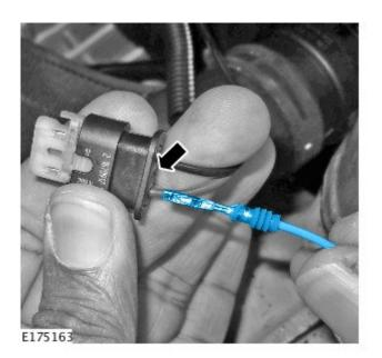
**7.** Install the anti-back out bar to the electrical connector C1E318.
