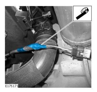
**15.** Install the electrical connector C1E318 to the charge air coolant pump.
