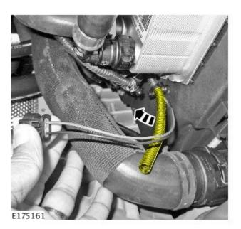
**5.** Release the anti-backout bar from the electrical connector C1E318.
