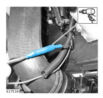
**13.** Install the outer harness protector to fully cover the crimped joint.
