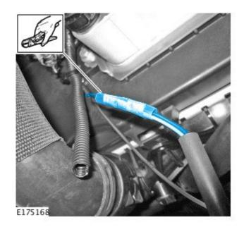
**12.** Install the glue-lined heat shrink into position to cover the crimp. Use a heat source to make sure the heat shrink is correctly bonded to the butt connector to form a water tight seal.
