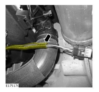
**14.** Install suitable electrical tape to secure the harness protector.
