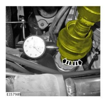
**6.** Mark the front driveshaft joint head relative to the axle for installation purposes.
