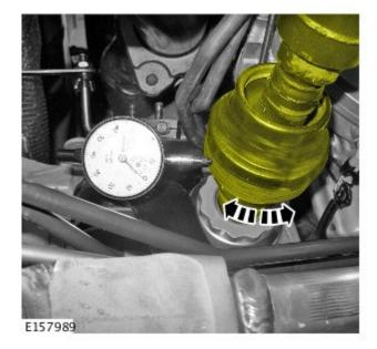
19. NOTE: make sure position of driveshaft joint is marked relative to the axle
