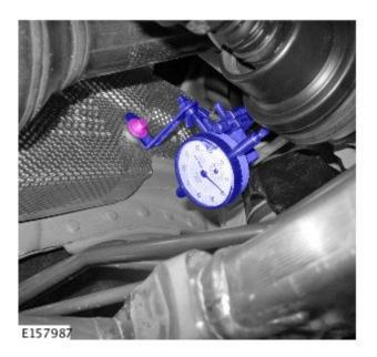
**4.** Position dial gauge pointer so that it is touching the surface of the inner front driveshaft coupling.
