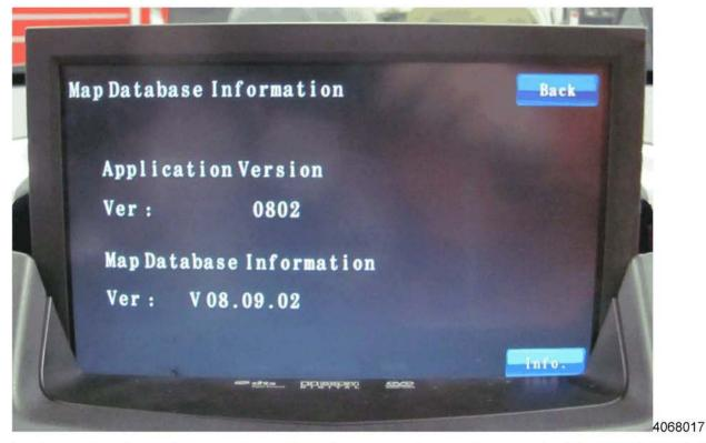
To determine the radio control module software version, navigate to the Map Database Information screen using the radio. Use the following navigation path: CONFIG>NAV>Map Database Information. Refer to the Application Version field on screen to determine the software version. Refer to photograph.
