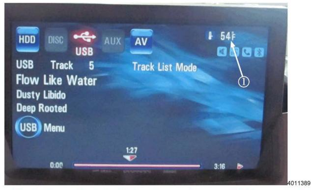
**Note:** The ignition must be in the RUN position to perform step 16. Make sure the HVAC is functional to check that you are in the RUN position. If you can't change the fan speed of the HVAC you are not in the RUN position.
