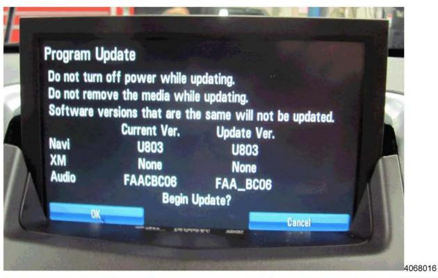
**Note:** The Download Complete screen appears and disappears in a short period of time. If you are not present when the screen appears, the Program Update screen appears. If the Program Update Screen appears and the current software version field and the update software version field are the same or None" or "Same" is listed in the software version fields, select "Cancel" and proceed to step 13.
