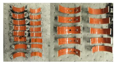
If both the main bearings and connecting rod bearings show no signs of significant wear (surface finish is not dull)
