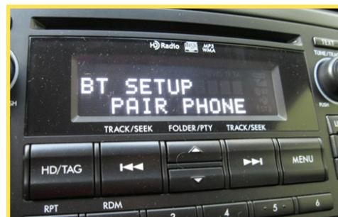
**NOTE:** If the system does not automatically display the **SETUP / PAIR PHONE** screen after the **WELCOME** screen refer to **TSB 15-186-15**
