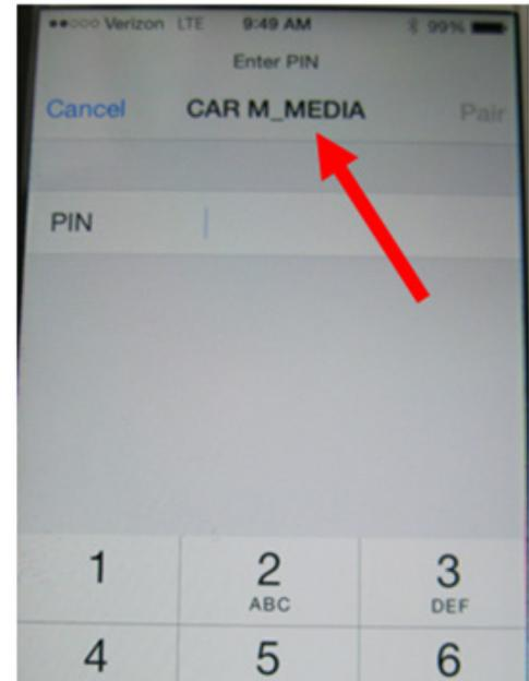
**IMPORTANT NOTE:** When pairing some Android-based phones, if unable to pair the phone, the pass key may need to be changed from the default 1-2-3-4 to 0-0-0-0. The pass key change can also be performed using the VR feature. Exit the pairing procedure by cycling the key then performing the pass key change steps listed below.
