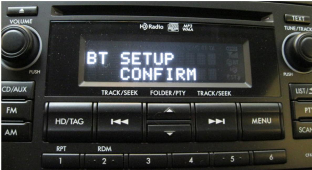
**Step 6.** After repeating “CONFIRM”, the system will automatically begin the pairing process and start searching for a phone to pair with. The system generates its own “name” which will be shown on the display and on the phone’s list of paired devices. In this case “CAR M\_MEDIA” was the name used.
