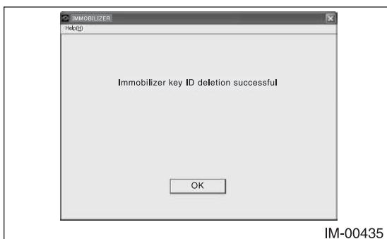
13) The screen shows that processes have been completed. Remove the key and click the [OK] button.
