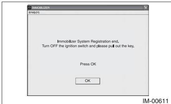
17) Make sure the engine can be started with all the registered keys, then quit the registration procedure.
