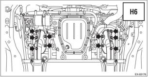
**CAUTION:** The front exhaust pipe assembly is heavy and the heat shield edges can be very sharp. Use appropriate personal protective equipment (PPE) and care while lifting.
