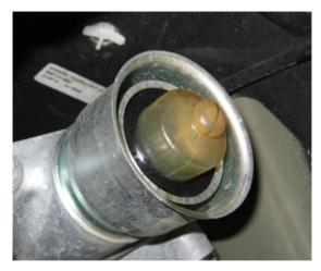
**IMPORTANT NOTE:** There will be a very small amount of CVT fluid that will drip out of the transmission and the slip yoke after removing it from the transmission. **Always** make sure to thoroughly clean any fluid residue off of the exhaust system and surrounding components.
