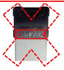
Never install a stop lamp switch with the "INFAC" logo stamped on the body in any of the vehicles covered by TSB SC098
