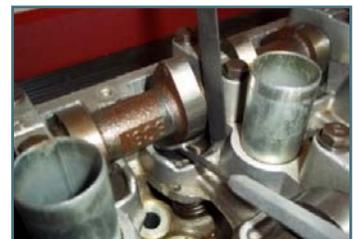
Once the shim is removed, measure its thickness with a micrometer. The chart on the next page is needed to make our calculation for the new shim to be installed. Looking at the valve adjustment chart provided in the Service Information for this vehicle (Figure 1), we must locate our measured valve clearance on the right side of the chart; our measurement in this example is 0.32mm as stated earlier.
