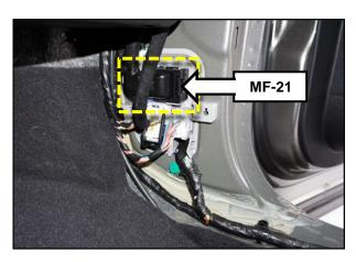
8. Use a small brush to apply Stabilant 22A to pins 47, 48 and 60, as shown. NOTE: Allow five (5) minutes of drying time after applying Stabilant 22A, prior to re-connecting the connector.
