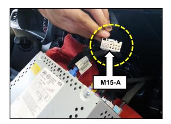
4. Carefully place the head unit on the bench and apply Stabilant 22A to the ten (10) small, male pins on the right side of the connector, as shown. NOTE: Allow five (5) minutes of drying time after applying Stabilant 22A, prior to re-connecting the connector.
