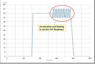
To complete the EGR Readiness Monitors for the Borrego (HM), technicians will need to road test a completely warmed up vehicle, above 45 mph, for several cycles, and under different loads (see below).
