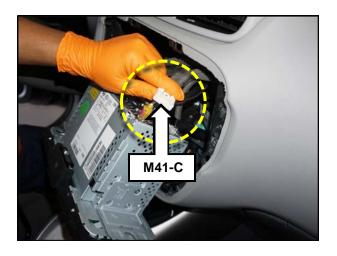
3. Carefully place the head unit on the bench and apply Stabilant 22A to all pins on connector M41-C, as shown. NOTE: Allow five (5) minutes of drying time, after applying Stabilant 22A, prior to reconnecting the connector.
