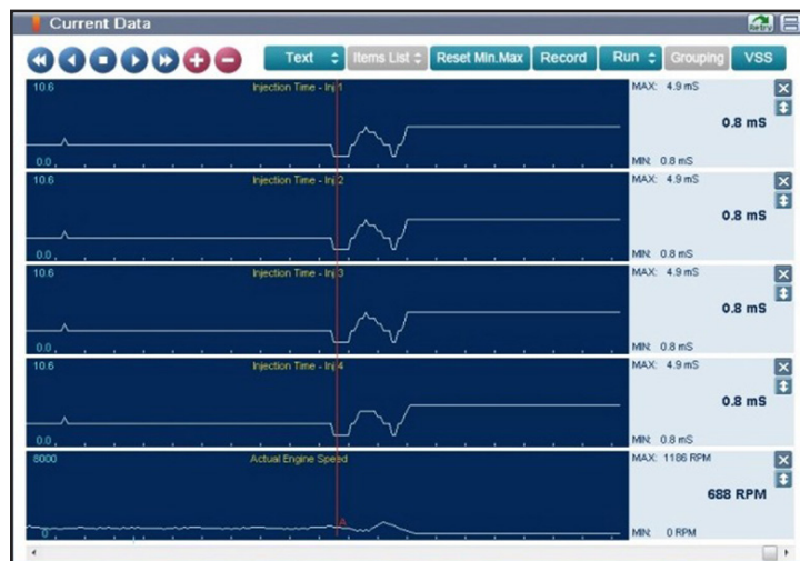
Fig. 4 Injector Pulse width reaction to a rich condition
