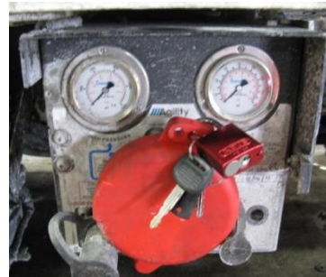
Figure 6 Lock-out the system as per your facility safety policies require. Removing the vehicle ignition key can be used to lock-out the fuel system.
