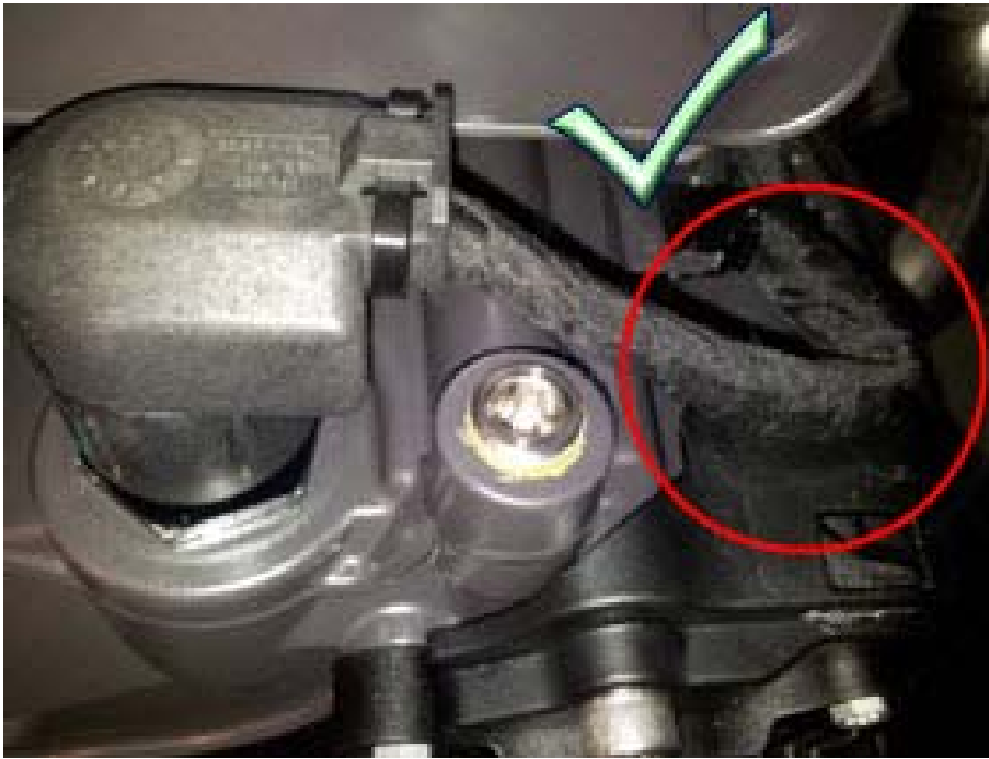
Front top harness incorrect routing
