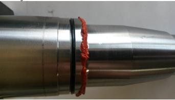
4) Press new stainless steel seal sleeve on to spindle with fingers until squarely seated.
