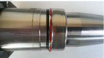
5) Use installation tool and hammer to drive stainless steel seal sleeve into position ensuring that stainless steel seal sleeve is not crooked on spindle.
