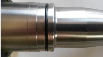
3) Apply liberal amount of high temperature red RTV silicone sealer to spindle seal sleeve journal surface.
