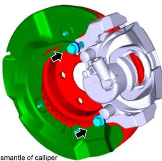
2- Remove the bolts w/o dismantle of calliper from anchor bracket
