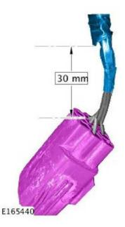
5. ONOTE: Make sure the protective sleeve is a minimum of 30mm from the electrical connector.
