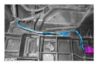
3. ONOTE: There must be a minimum of 30mm between the connector and the end of the bumper harness protective sleeve.
