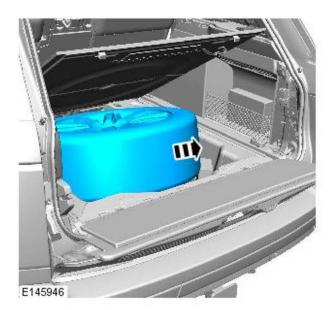
NOTE: The air compressor unit is protected by an acoustic box which tilts to allow access to the vehicle battery.
