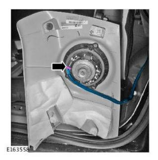
**5.** Using suitable cables ties, secure the filter wiring harness to the main vehicle harness.
