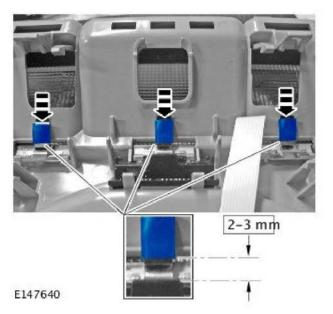
7. ONOTE: Do not damage the printed circuit
