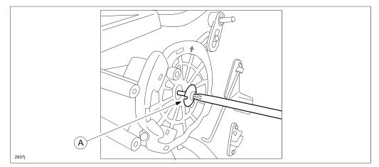
h. Rotate the air flow mode main link (A) several times back and forth between the "VENT" and "DEF" positions to verify the mode can be switched properly.
