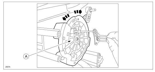
i. Rotate the air flow mode main link back and forth several more times to allow the grease to spread.
