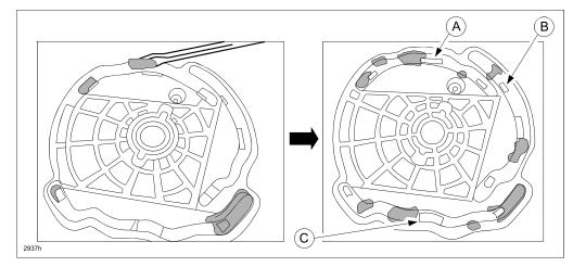
f. Install the air flow mode main link (with marked arrow (A) pointing upward) and engage the link for each mode door into the respective air flow mode main link channel.
