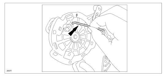
c. Remove the screw (A), then remove the air flow mode main link (B).
