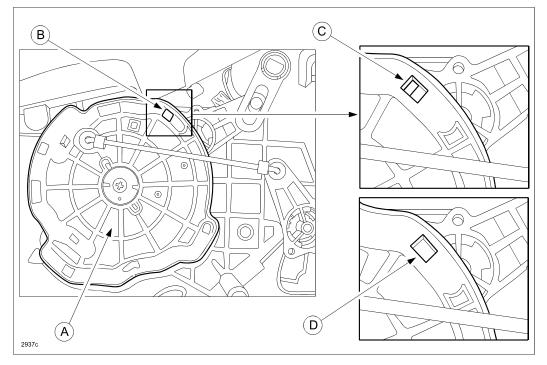
5. Remove the E-ring (A) at the tip of the mode selector wire and reinstall it to a maximum of 2 mm away (B) from the original position (C), as shown below.
