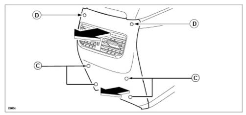
3. Re-install the rear console lid pin(s) back to the original position.
